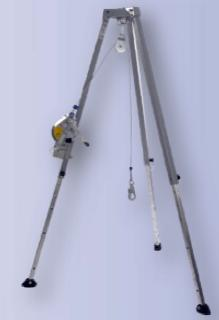
Under normal working conditions the system offers fall protection with the HRA device acting similar to a car seat belt. The life line is kept under constant tension by means of a self retracting cable drum. However, should a fall occur the automatic locking system will activate and an internal brake disk will absorb energy to well below the 6kN limit required by the EN 360 standard.
